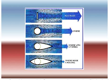
The shape of an object greatly influences aerodynamic drag/friction/resistance.
